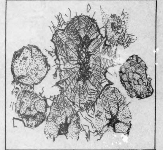
FIGURE 9. SPHERULITIC OOLITES, DEFORMED AND ALIGNED. Growth aprons extend into matrix. At left two undeformed pebbles of dolomite. Spec. 436, ac section, deformation 30 per cent. Beekmantown, a mile west of Mercersville, Md.
